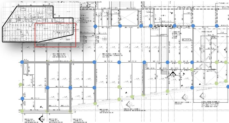
**Figure 7:** Level 3 framing plan showing hangers and outline of hung/cantilevered portion of building (S-103)
