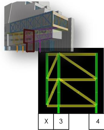
**Figure 32:** Truss J Location and Load Path Orientation
