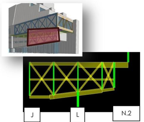
**Figure 30:** Truss X Location and Load Path Orientation
