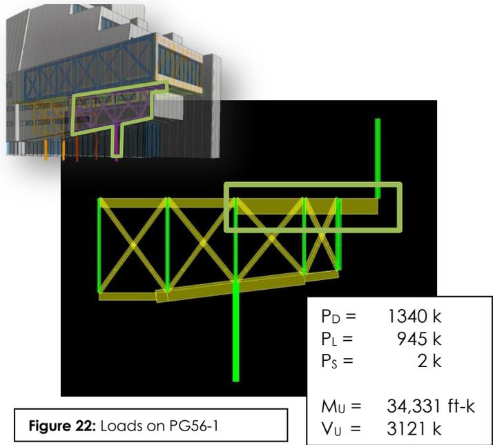
PG56-1 has the largest web thickness, the widest flange width, and the largest flange thickness of any established or proposed plate-girder cross sections. Though PG56-1 is designed adequately for the loads, this departure from precedent component plate dimensions could lead to adverse effects during fabrication and construction. These effects are explored further in the Construction Management Considerations section of the Final Report.
