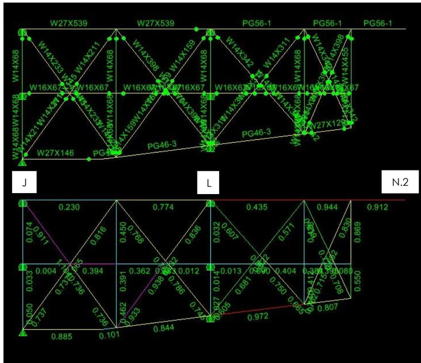
**Figure 31:** Truss X Modelina input and Design Results
