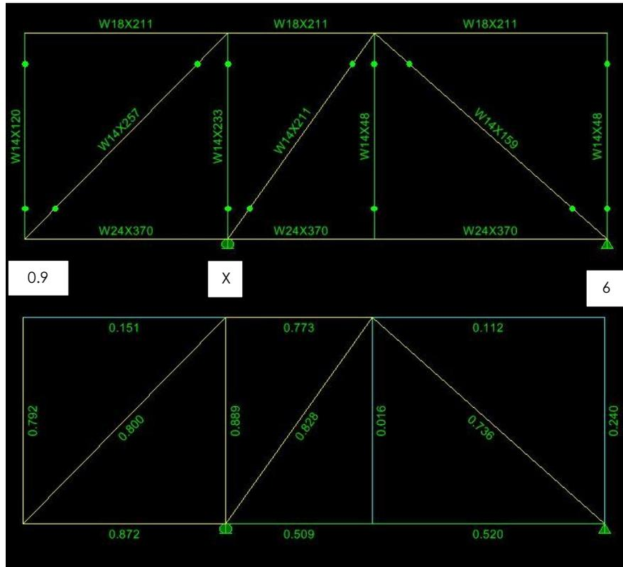
**Figure 29:** Truss N.2 Modeling input and Design Results
