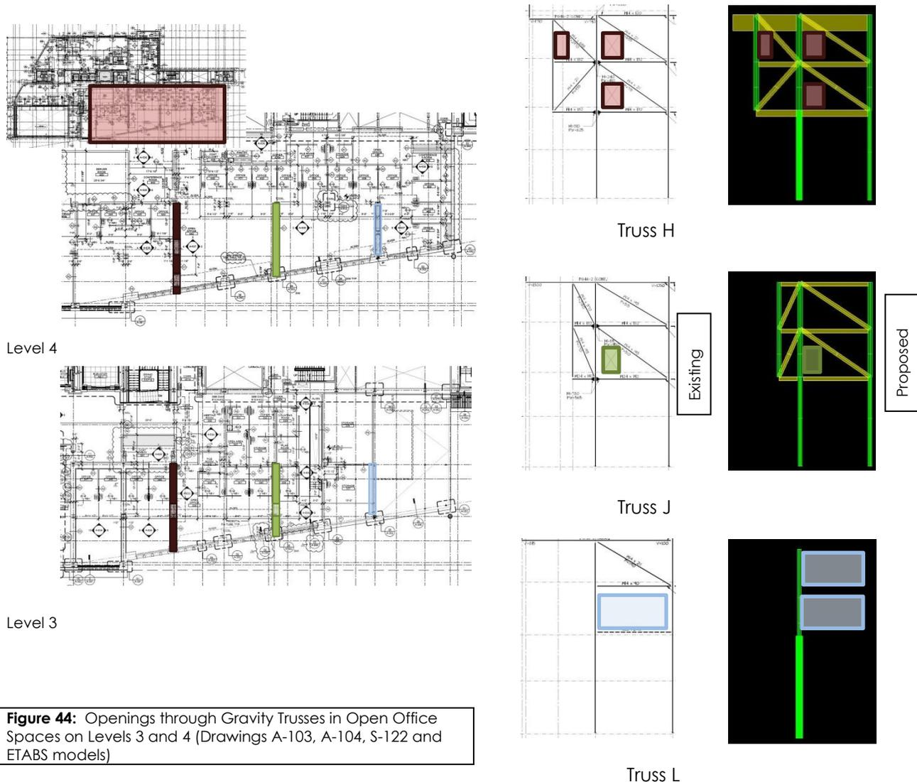
**Figure 44:** Openings through Gravity Trusses in Open Office Spaces on Levels 3 and 4 (Drawings A-103, A-104, S-122 and ETABS models)
