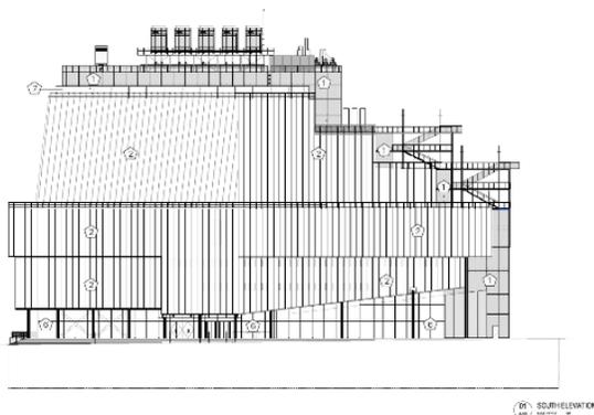
**Figure 3:** South Elevation showing modular façade (A-007)
