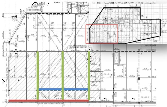
**Figure 6:** Level 3 framing plan showing transfer girders and lateral braced frames (S-103)
