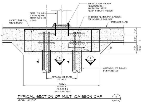
A pressure slab and the perimeter secant-pile walls operate in tandem to hold back the soil and groundwater below grade during construction and for the lifespan of the building. The walls vary between 24" and 36" and are set on 6'-6" wall footers and caissons. These are isolated from the pressure slab shown in Figure 4. Hydrostatic uplift led the engineers to design a 24" pressure slab, isolated from the 5" architectural slab-on-grade by a 19" layer of gravel.
