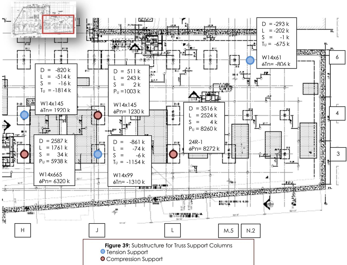
The loads shown in Figure 39 were used to analyze the capacity of the current pile arrangements before a final proposal could be issued. The capacities of assigned pile identifications are shown in Figure 40 below.
