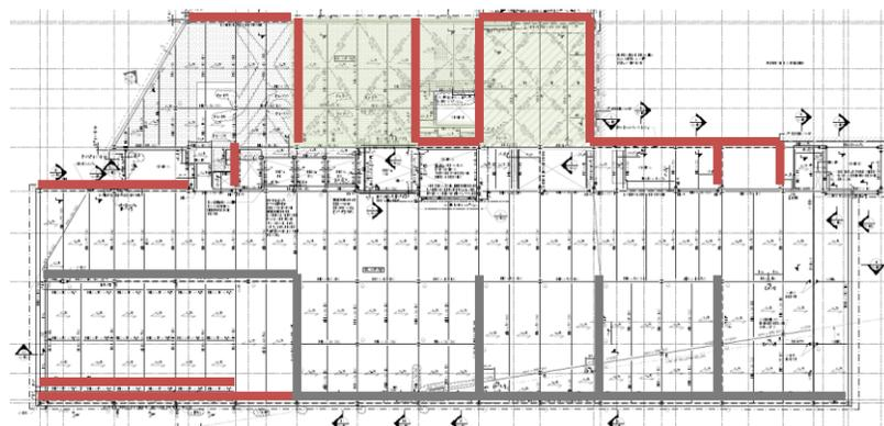
**Figure 9:** Level 5 Framing Plan Showing Lateral System (S-105)
