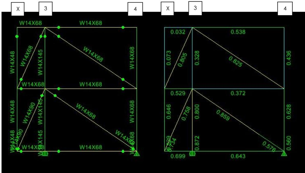
**Figure 33:** Truss J Modeling Input and Design Results
